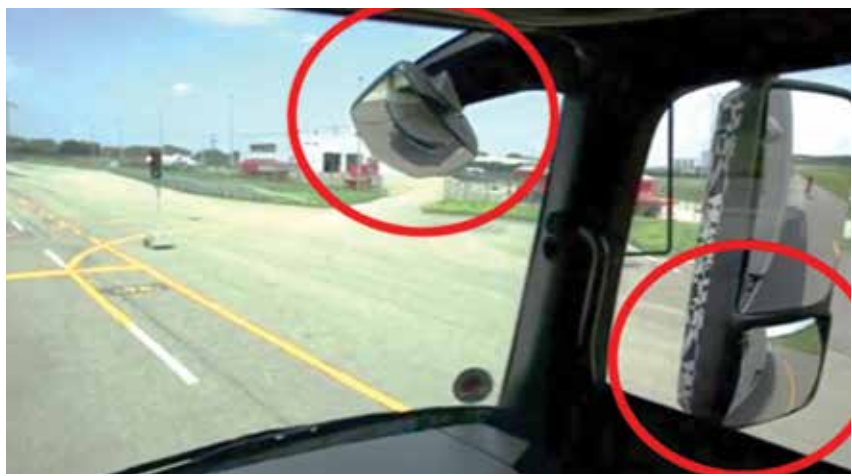
Figure 10.1: Internal mirrors installed in buses to cover blind spots Source: JPRI Kolkata City Accident Study)
