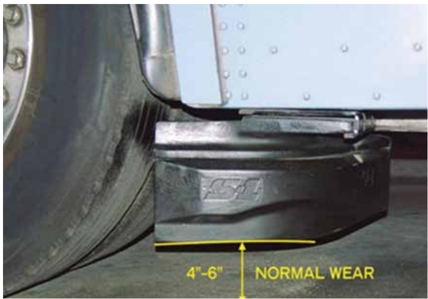
Figure 10.2: S1 Guard - Run-over Prevention Device
